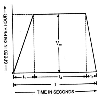
Let  $\alpha = \text{Acceleration in kmphps}$   $\beta = \text{Retardation in kmphps}$   $V_m = \text{Crest speed in kmph}$  T = Total time of run in seconds.Time for acceleration in seconds,  $t_1 = \frac{V_m}{\alpha}$ Time for retardation in seconds,  $t_3 = \frac{V_m}{\beta}$
